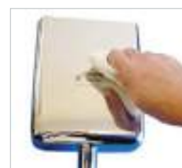
4. Clean etching area thoroughly using demineralised water
