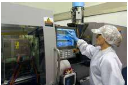
Highly trained operators monitor the moulding process
