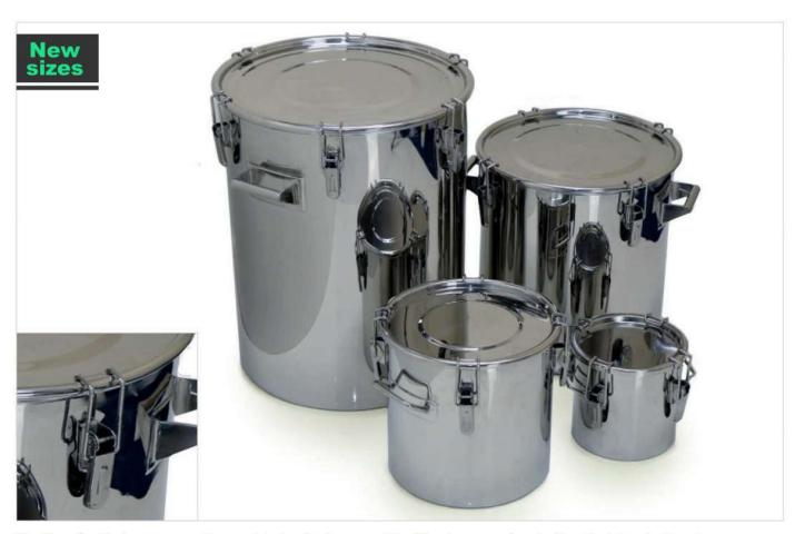
The Sampling Systems range of heavy duty toggle drums are ideal for storage and production. Each Toggle Drum is supplied with a fully welded handle, silicone seal (FDA grade) and lid. The lid is secured by using the pull down latches (toggle clamps). They are manufactured from high grade 316L stainless steel which makes the containers suitable for most applications.
