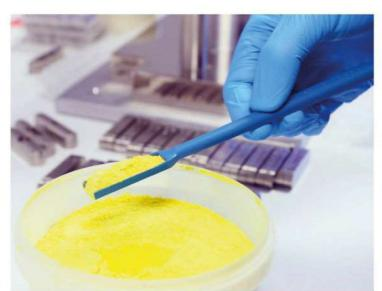
The Metal Detectable Micro-Spatula is ideal for sampling small volumes. Its narrow sampling blade enables samples to be taken from very small containers such as vials.
