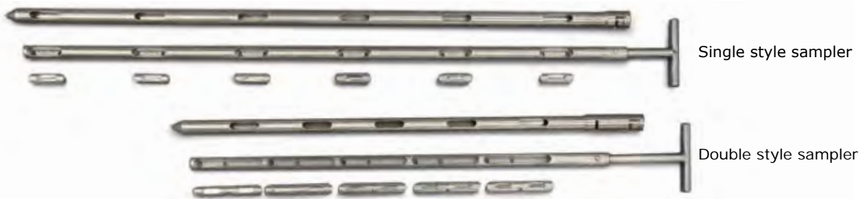
More than one sample can be taken from the same sampling point (see double or triple styles).
